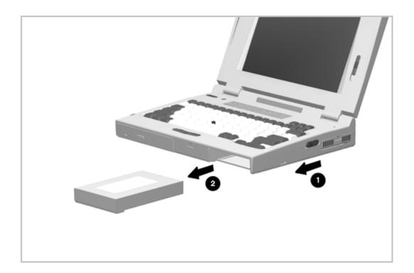
Figure 5-5. Removing the Battery Pack
